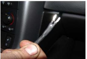
Figure 6: Fuse tap with marking
