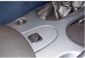
Figure 7: round lighted switch installed
