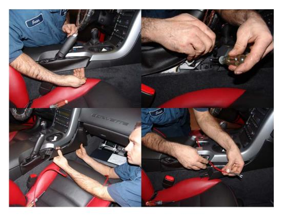
Figure 2: Removal of parking brake boot and side trim panel.
