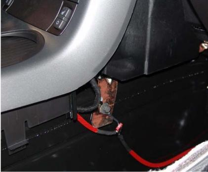
Firgure 4: Installing the ground strap
