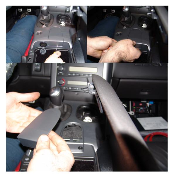
Figure 1: Removal of center console piece
